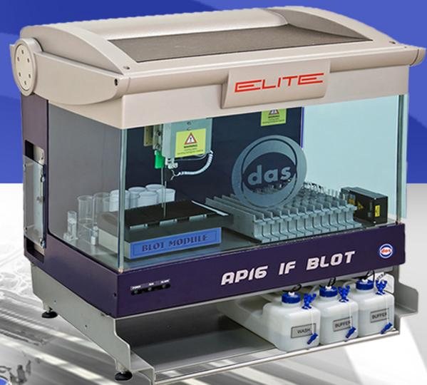
**AP16 IF ELITE** is an innovative and fast processor able to run 16 IFA slides with any kind of thickness, mask, well shape and number of rows. It is equipped with a sliding-sample barcode reader and a camera for slide barcode reading. Reliable and manufactured with the latest technologies, it is able to carry out: sample dilution, sample and reagent dispense, different incubation times and slide well different washing types with accuracy and precision.
